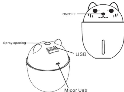
Turn counterclockwise and unscrew the top cover. Fill the tank with water (320ml). Unscrew the top cover clockwise and connect the power supply (USB cable). Click on the button (nose) to start the humidifier.
